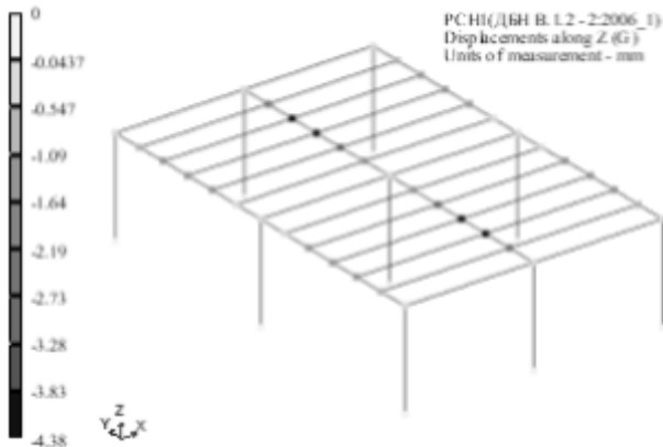
Fig. 7(a). The results of the static analysis of the building (displacements by Z) before the fire
